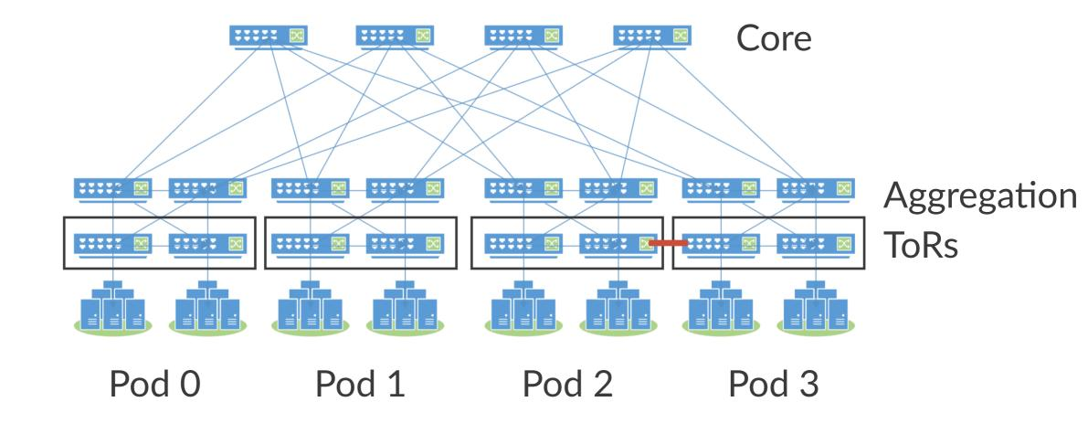
"The pair between the last ToR in the last third pod and the last ToR in the penultimate pod"
