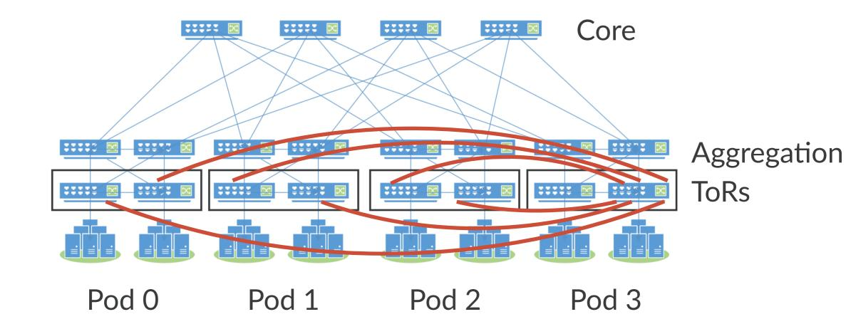
"The pairs between the last ToR in the penultimate pod and the ToRs in the last pod (except the last ToR, which is included in the last case)"
