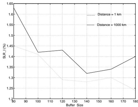
Figure 9.19 - Slice Loss Ratio (I Frame) vs link distance
