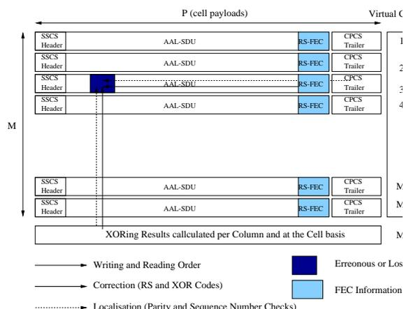
Figure 3 - Virtual Matrix of Control Blocks
