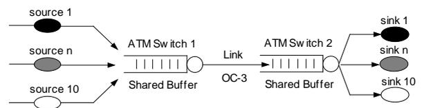
Figure 6 - Network Simulation Model
