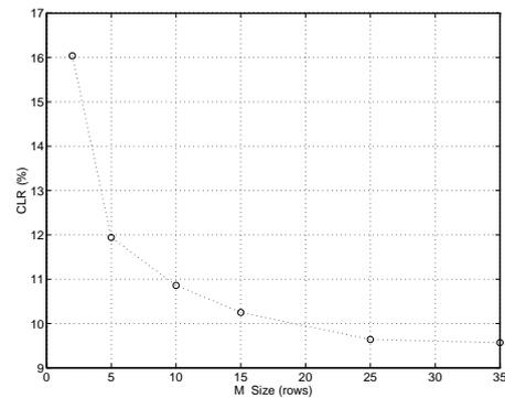
Figure 9.22 - Cell Loss Ratio vs Data Redundancy Ratio (Aggregate Stream)
