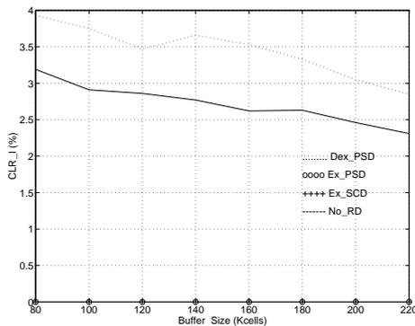
Figure 9.2 - Cell Loss Ratio (I Frame)
