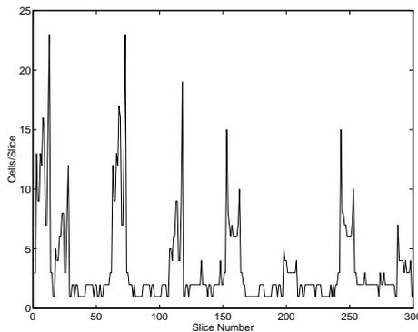
Figure 7 - Number of ATM cells per slice for the first 20 frame of the MPEG-2 video sequence.
