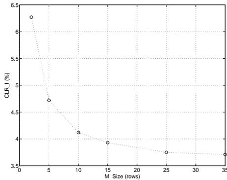
Figure 9.23 - Cell Loss Ratio vs Data Redundancy Ratio (I Frame)
