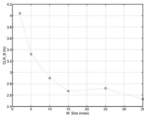
Figure 9.25 - Cell Loss Ratio vs Data Redundancy Ratio (B Frame)
