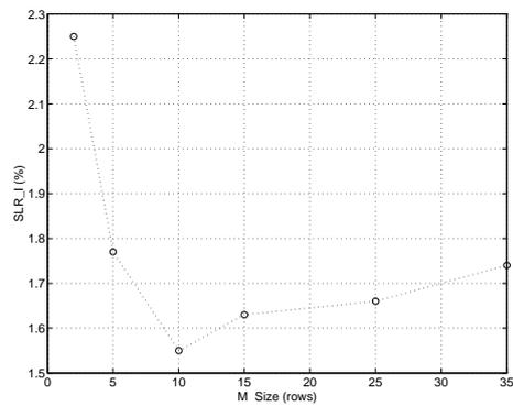
Figure 9.27 - Slice Loss Ratio vs Data Redundancy Ratio (I Frame)
