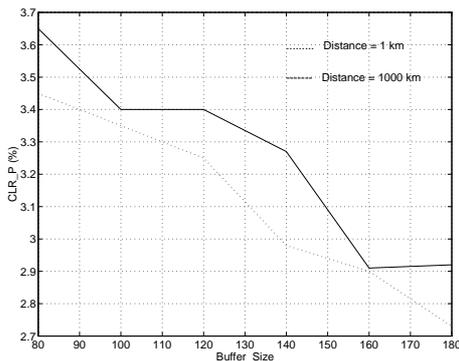
Figure 9.16 - Cell Loss Ratio (P Frame) vs link distance
