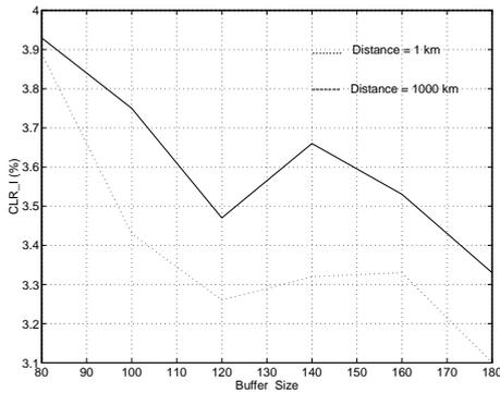
Figure 9.15 - Cell Loss Ratio (I Frame) vs link distance
