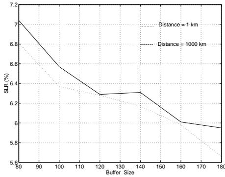
Figure 9.18 - Slice Loss Ratio (Aggregate) vs link distance
