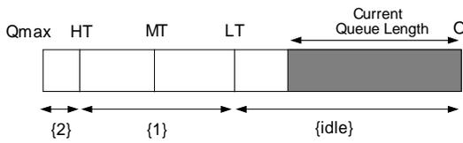
Figure 4 - SA-PSD operation modes
