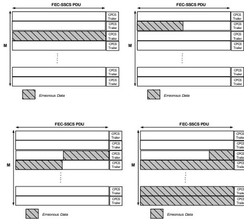
Figure 5 - Cell Loss Distribution using SA-PSD
