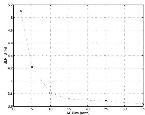
Figure 9.29 - Slice Loss Ratio vs Data Redundancy Ratio (B Frame)
