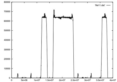
Figure 9.8 - Buffer Occupancy with Ex-PSD
