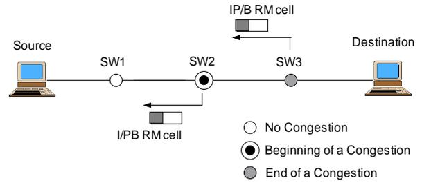
Figure 1 - DexPAS Operation with Transmission of RM cells
