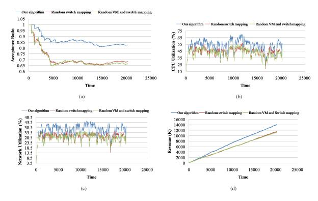
Fig. 4. Comparison of acceptance ratio, resource utilization and revenue over time for VDC requests of VL2 topology. (a) Acceptance Ratio. (b) CPU Utilization. (c) Network Utilization. (d) Revenue
