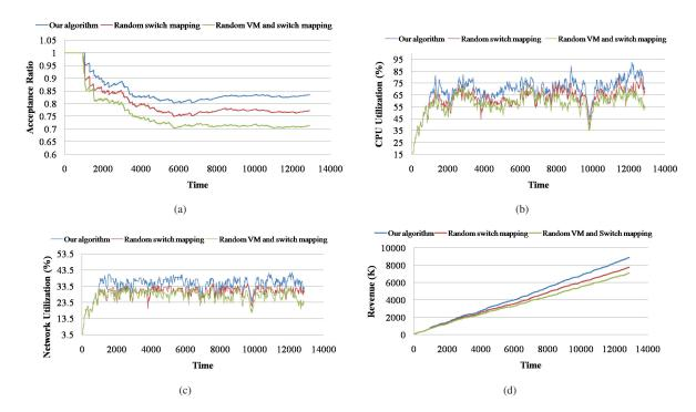
Fig. 5. Comparison of acceptance ratio, resource utilization and revenue over time for VDC requests of mix of VL2 and star topology. (a) Acceptance Ratio. (b) CPU Utilization. (c) Network Utilization. (d) Revenue
