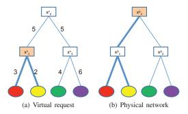
Fig. 2. Minimizing communication cost
