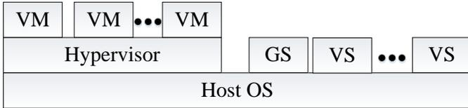
Fig. 3. Software stack of a DOT node
