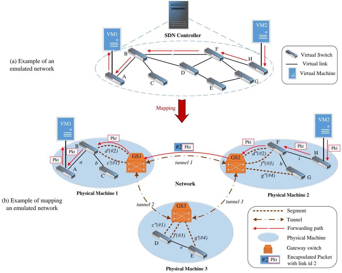
Fig. 4. Emulated network embedding and traffic forwarding in DOT
