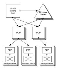
Figure 1. The Policy-Based Networking basic schema
