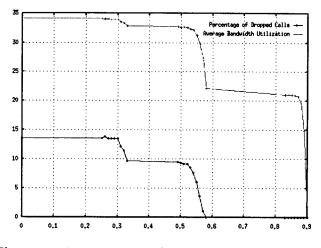
Figure 2: Average bandwidth utilization and percentage of dropped calls, Distributed CAC case
