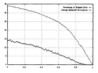
Figure 3: Average bandwidth utilization and percentage of dropped calls, random admission case
