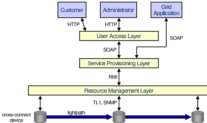
Figure 1. High-level architecture of the lightpath management system.
