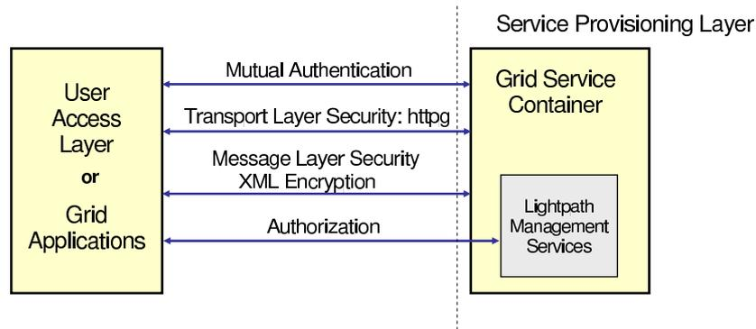
Figure 2. Security Mechanisms in the lightpath management system
