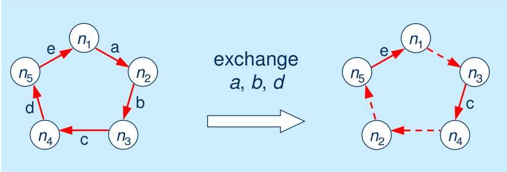
Figure 6: Example 3-branch exchange operation in a unidirectional ring. The operation changes the order of nodes in the logical topology.
