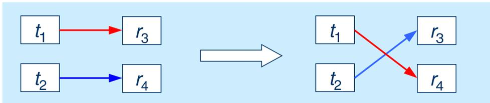
Figure 3: Example branch exchange operation in a multi-hop broadcast network among transmitters  $t_1, t_2$  and receivers  $r_3, r_4$ . Solid arrows indicate unidirectional logical links, each using a dedicated wavelength.
