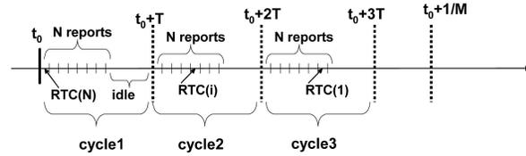
Fig. 6. Transmission cycles in the unsaturated regime.
