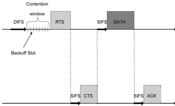
Fig. 4. Basic access mechanism of the IEEE 802.11 DCF.
