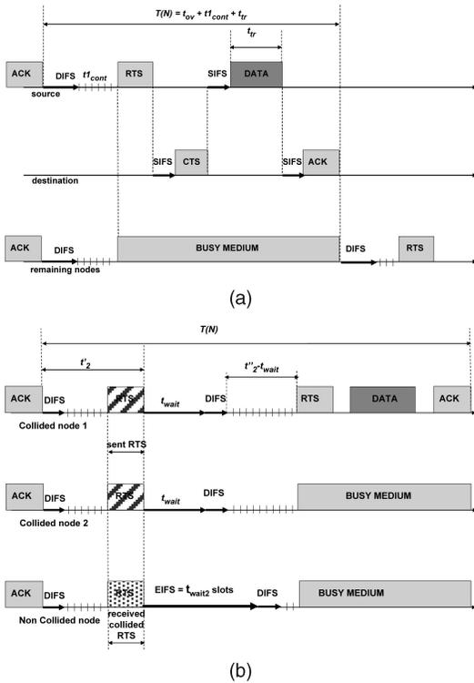
Fig. 5. The RTC. (a) Successful transmission from the first attempt. (b) Successful transmission after a first failed attempt.
