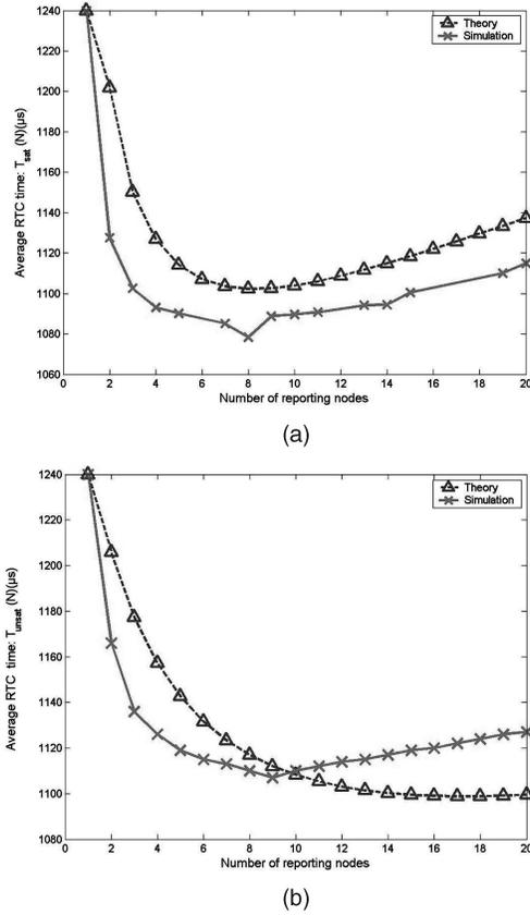
Fig. 9. Average time to report an event (i.e., the RTC). (a) Saturated regime-case:  $T_{sat}(N)$ . (b) Unsaturated-regime case:  $T_{unsat}(N)$ .
