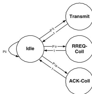
**Fig. 7** Markov model of wireless transmission
