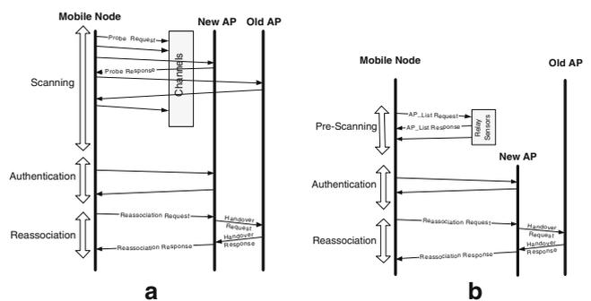
Fig. 5 a Handoff process. b Fast handoff using sensor networks
