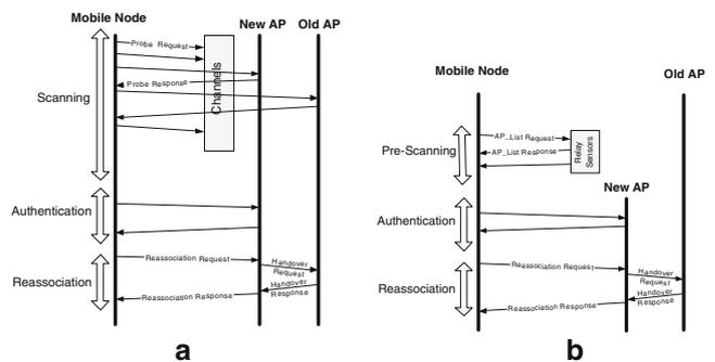
Fig. 5 a Handoff process. b Fast handoff using sensor networks
