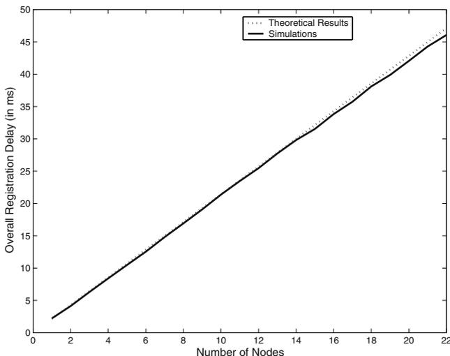
**Fig. 9** Registration delay (theoretical results validated through simulations)
