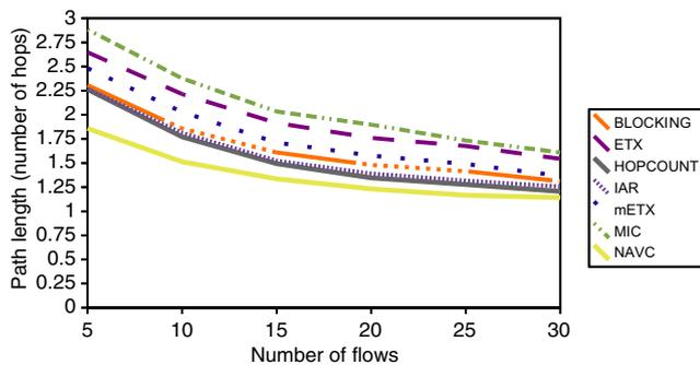
**Fig. 10** Number of hops with increasing number of flows for a 50-node network
