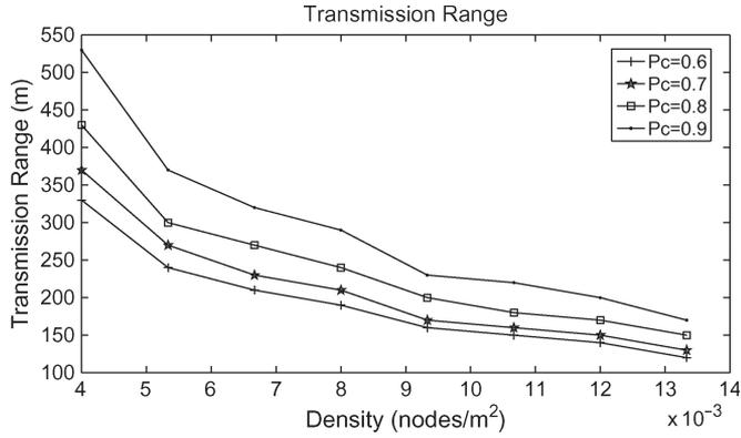
Fig. 3. Transmission range as a function of node density.
