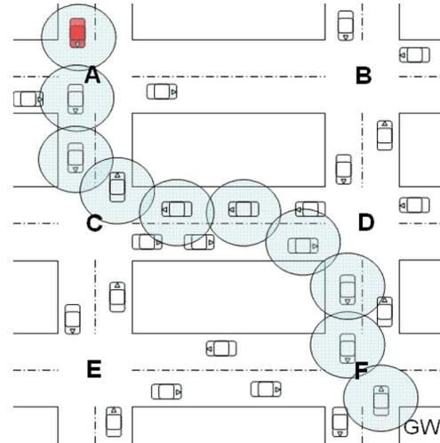
Fig. 1. Message routing in VANETs using IGRP.
