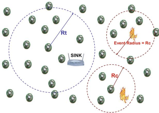
**Fig. 1** Typical sensor network topology with event and sink.  $R_t$  is the transmission range of each sensor.  $R_c$  is the sensing range of each sensor. All the nodes that are within the event range  $R_c$  are able to detect the event. The sink is interested in collecting information from sensor nodes within the event radius  $R_c$
