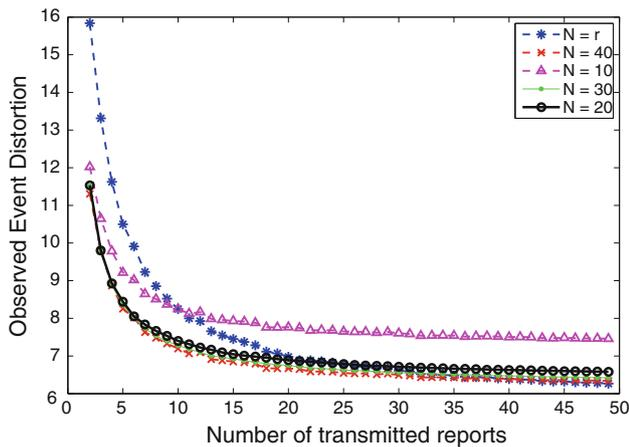
**Fig. 2** Average distortion as a function of the number of transmitted reports considering different values of active reporting nodes
