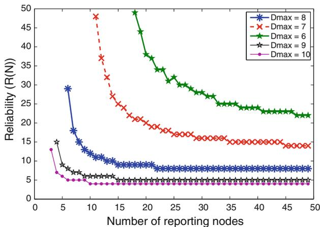
**Fig. 3** Average reliability as a function of the number of reporting nodes for different distortion values
