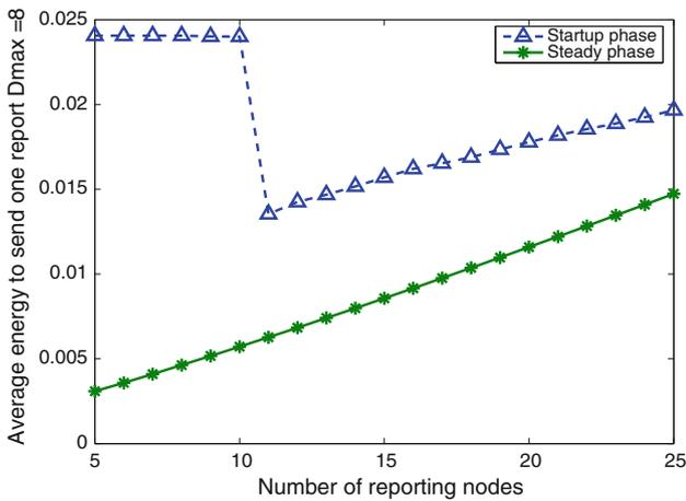
**Fig. 18** Average energy to send one report during both phases: startup and steady: case  $D_{max} = 8$
