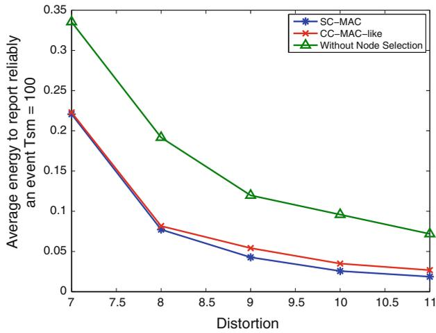
Fig. 22 Comparison of the energy consumption among SC-MAC, CC-MAC and without node selection protocols
