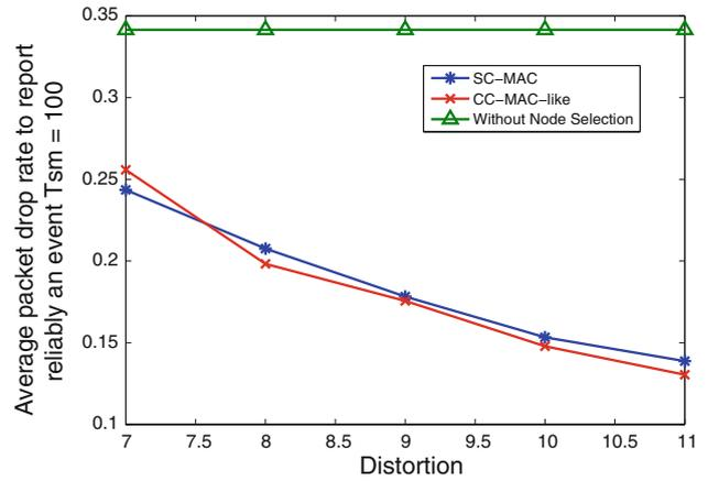
Fig. 24 Percentage of dropped packets for the three MAC protocols
