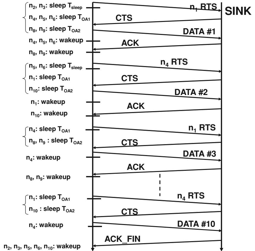
The steady phase continues until the reception of an ACK\_FIN by the reporting nodes from the sink. The ACK\_FIN indicates that  $R(N_{opt})$  reports are already received by the sink node. In Fig. 10, the messages exchanged during this example are shown.
