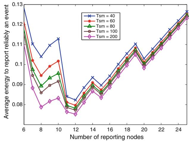
**Fig. 19**  $T_{sm}$  impact on the energy consumption: case  $D_{max} = 8$
