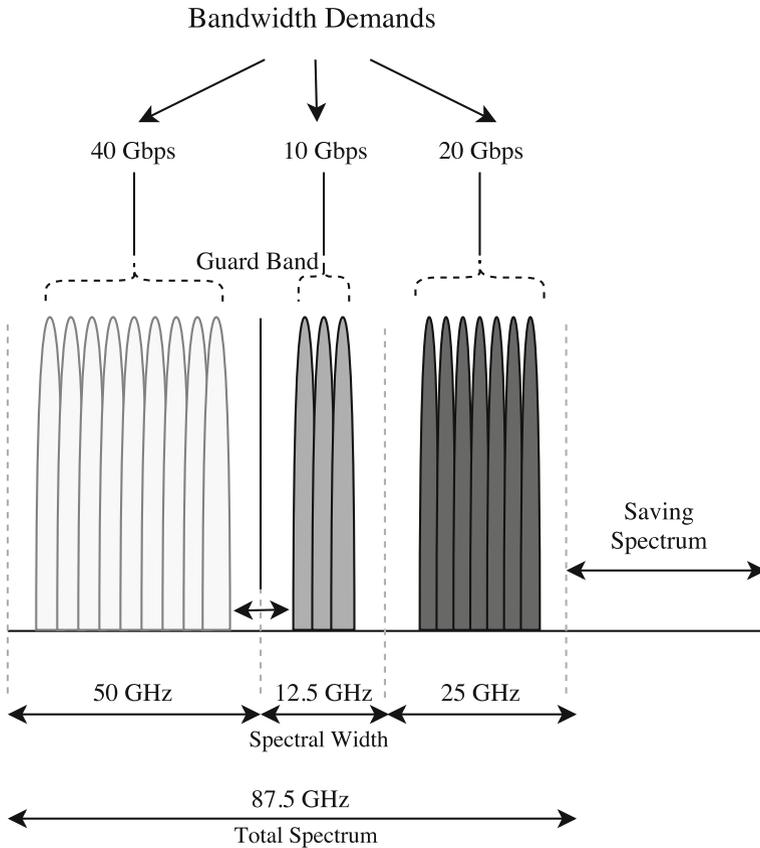
**Fig. 4** Spectrum allocation in an EON
