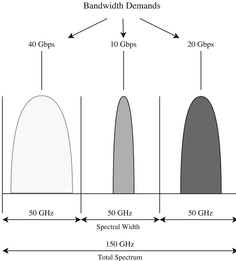
**Fig. 3** Spectrum allocation in a fixed-grid network
