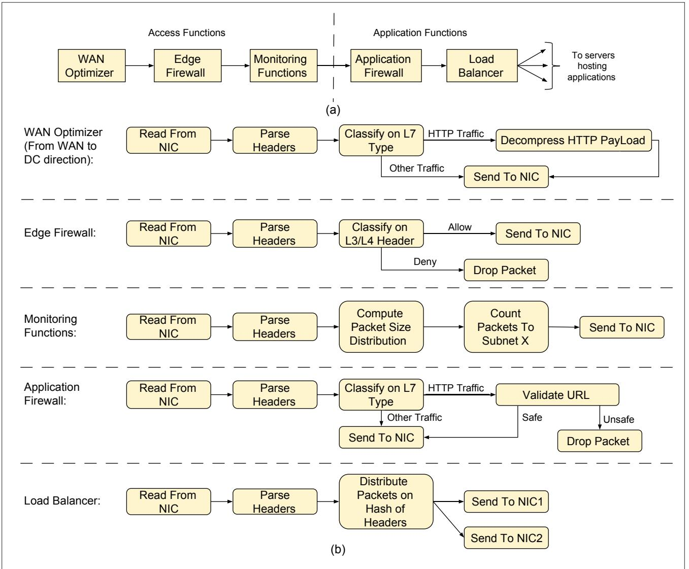
FIGURE 2. Illustrative example to motivate microservice-based VNFs: a) example SFC for data center networks; b) functional decomposition of the VNFs in Fig. 2a.
