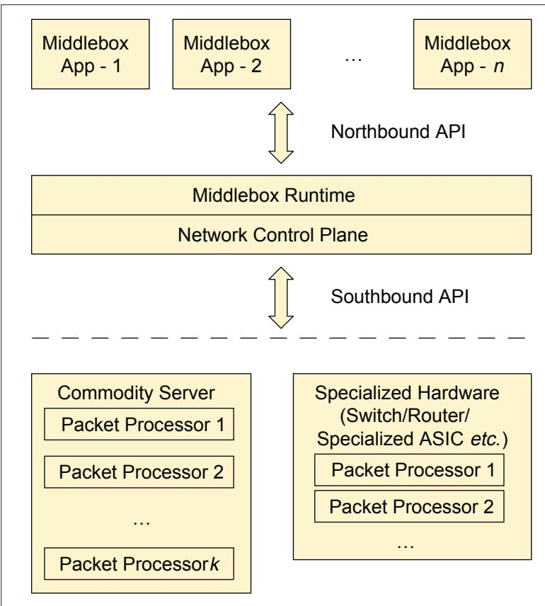
FIGURE 4. Generalized architecture of OpenBox [8] and Microboxes [9].
