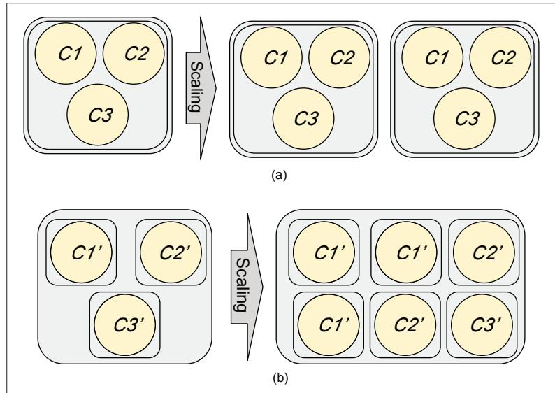
FIGURE 1. Monolithic vs. microservice-based application: a) a monolithic application with tightly coupled components, inefficient scaling and coarse grain resource allocation; b) a microservice-based application with independently scalable microservices, facilitating fine grain resource allocation.
