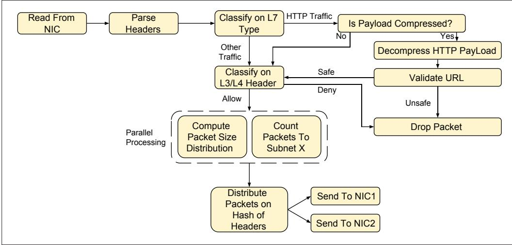
FIGURE 3. Microservice-based realization of the SFC in Fig. 2a.
