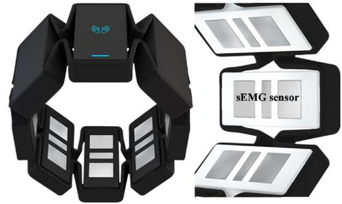
Fig. 5. Myo armband and its integrated sEMG sensors.
