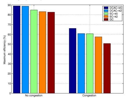
Fig. 12. Maximum efficiency for load = 150.
