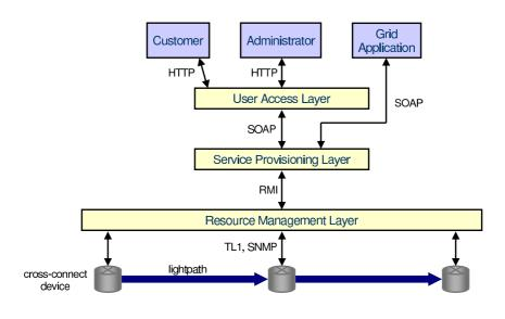
Figure 1. High-level architecture of the lightpath management system.
