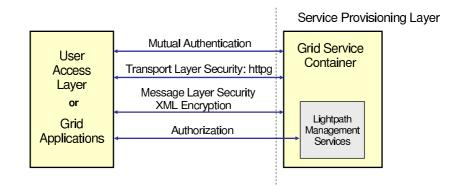
Figure 2. Security Mechanisms in the lightpath management system
