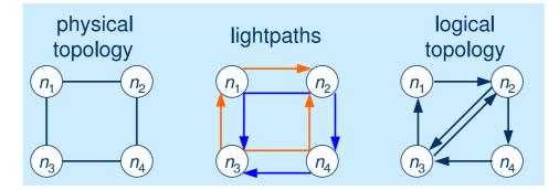
Figure 2: Example optically switched ring network and configuration. Each node is equipped with two transmitter/receiver pairs. Each fibre is bidirectional and carries up to two wavelengths. The logical topology shown has been optimized for bidirectional traffic between nodes  $n_2$  and  $n_3$ .
