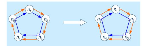
Figure 5: Example merge operation to establish a lightpath from node  $n_1$  to node  $n_4$  in a unidirectional ring. The inverse operation can be used to establish a lightpath from  $n_2$  to  $n_4$ .
