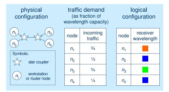
Figure 1: Example single-hop broadcast WDM network and configuration.
