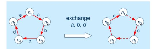
Figure 6: Example 3-branch exchange operation in a unidirectional ring. The operation changes the order of nodes in the logical topology.
