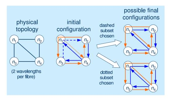
Figure 4: Example subset selection in Path-Add heuristic with K = 1 and L = 2. The dashed and dotted subsets of lightpaths in the initial configuration are considered for deletion in order to establish a lightpath from  $n_1$  to  $n_2$ .
