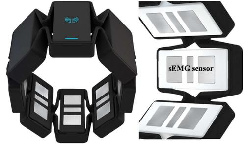
Fig. 5. Myo armband and its integrated sEMG sensors.
