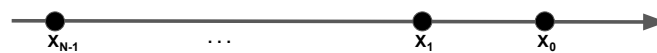
Figure 3. Vehicle i 's position on the one directional link is shown with x_i . The first vehicles is indexed 0.
